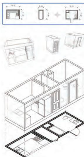
Repetitive core components, designed for modular prefabrication and enhanced energy performance, can be used in multiple configurations for the design of new infill housing and the retrofit of existing homes.
