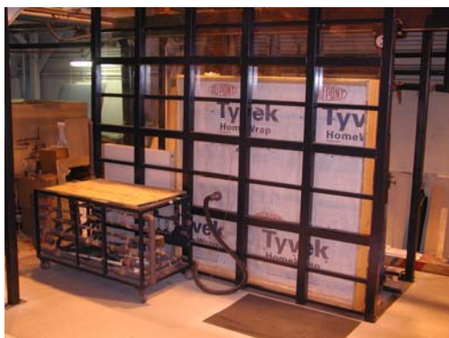
All Purpose ( \Delta_t , \Delta_p , rain) Test Rack
