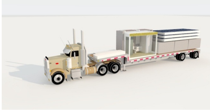
Figure 3: View of a Solar Thermal Full Bath REEM and a Solar PV Carport REEM as modular components on a single flatbed trailer.
