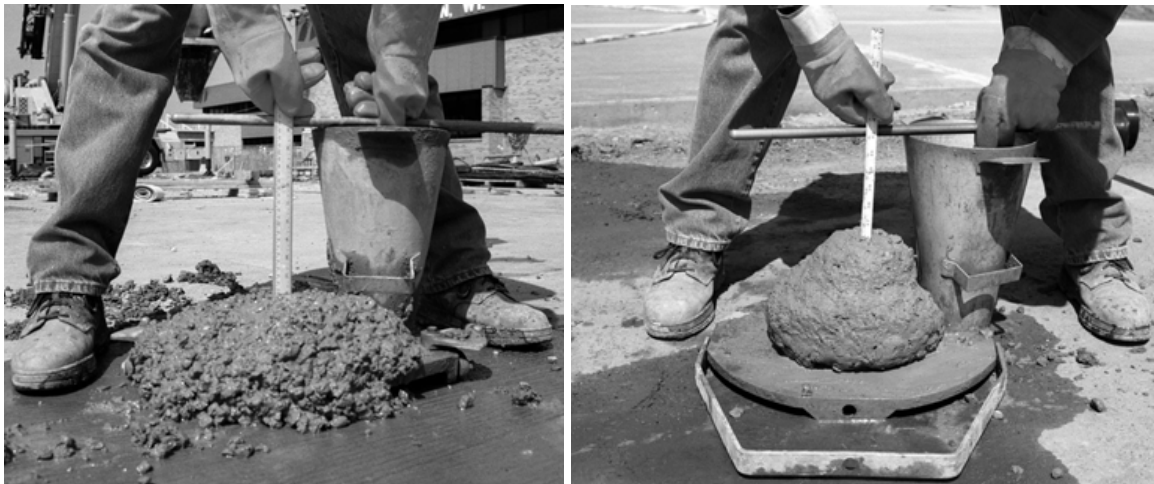
Figure 2. Slump test (left: High slump; right: Low slump)
