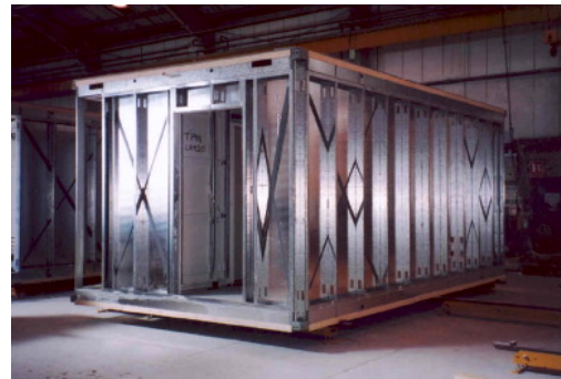
Figure 3. Load Bearing Wall 3D Module (image by Lawson and Ogden, 2008)
