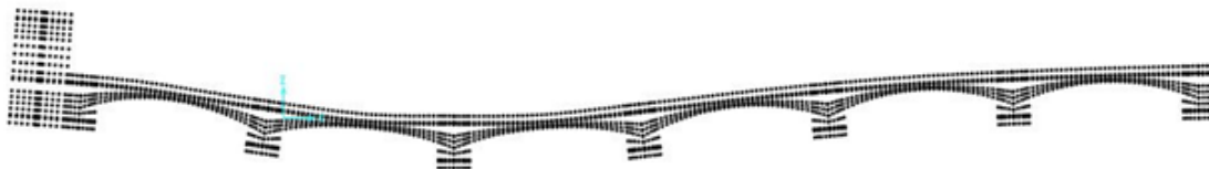
Figure 7: Deflected Shape in X-direction at Stage 2, magnified 50x for illustration
