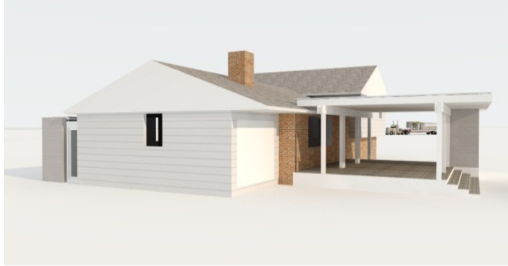
Figure 10: View of REEMs attached as saddlebags to a typical split-level house without obstructing the existing roofline.
