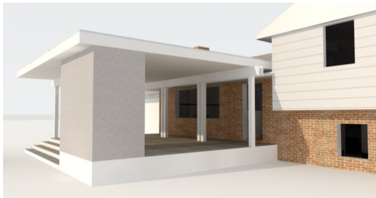
Figure 11: View of Solar PV REEM attached to a new deck platform and overlapping the existing house roof without physical attachment.
