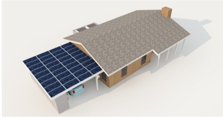
Figure 5: Aerial view of a typical 3 bedroom, 1 bath ranch house with a Solar Thermal REEM added as a full bath to the rear and a Solar PV REEM added as a carport to the side.
