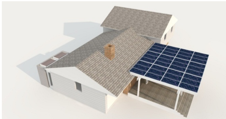
Figure 9: Aerial view of a typical 3 bedroom, 1 bath split-level house with a Solar Thermal REEM added as a laundry room to the rear and a Solar PV REEM added as a porch to the front.
