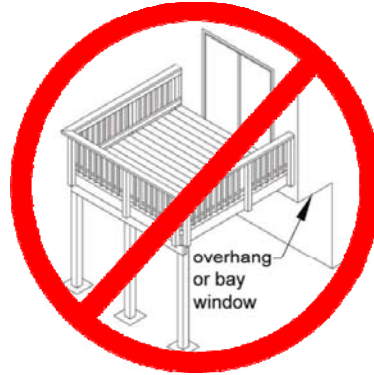
Figure 18. No Attachment to House Overhang
