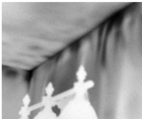
Attic air infiltration into the wall
