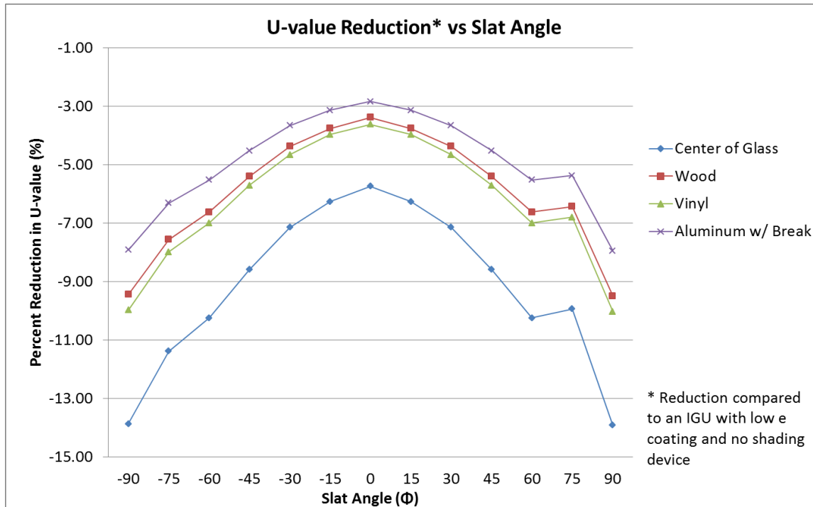
Figure 4: Reduction in U-value vs. slat angle.
