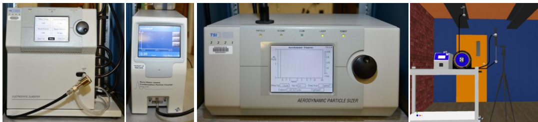
Figure 1. a. Schematic diagram of the field experiment at the MorningStar Solar Home; b. Particle sizing units that will be used to measure real time particle size distributions from 0.02 to 20 microns within the ductwork; c. Spatial profiling particle sizing set up.
