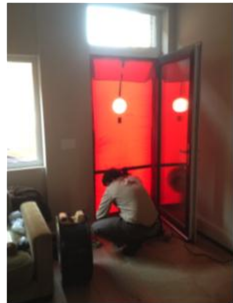
Figure 16: Photo of blower door test for first completed unit, with measured results
