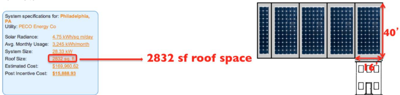
Figure 2, Required roof area for 20.5 kWh/sf/year consumption
