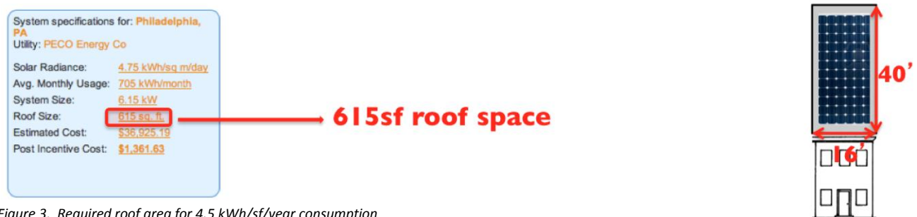
Figure 3, Required roof area for 4.5 kWh/sf/year consumption
