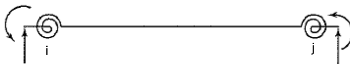
Fig. 2 Frame Element with Semi-Rigid Connections
