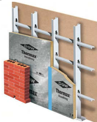
Figure 24 Section of THERMAX™ Sheathing (Courtesy of the Dow Chemical Company)
