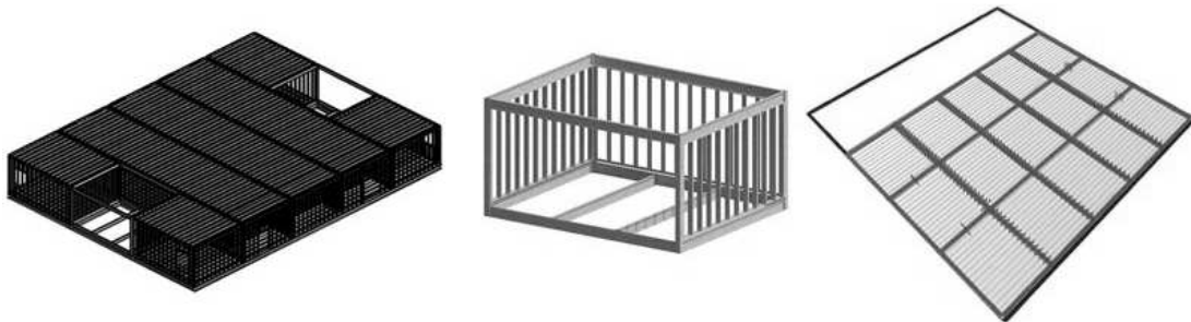
Figure 6. (a) Rendering of the wall-bearing single-story expansion used in the study (b) Conceptual maintenance module envisioned to house roof-top mechanical equipment servicing the existing building (c) The finite element model of the steel beam transfer grid.
