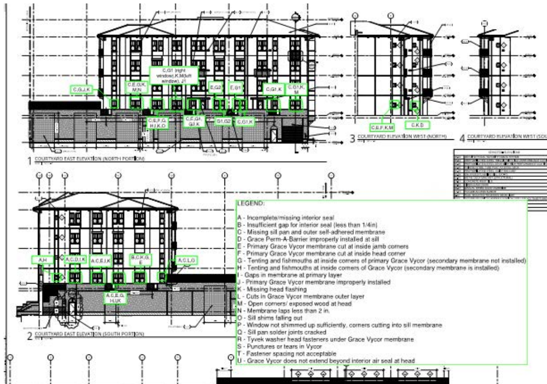
Figure 9. Case Study #1: Example elevation documenting the required extensive field repairs to the factory installed window installations
