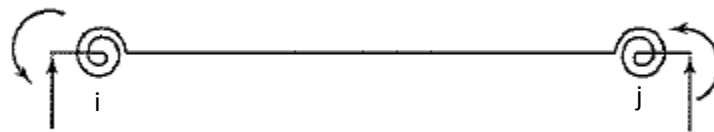
Fig. 2 Frame Element with Semi-Rigid Connections
