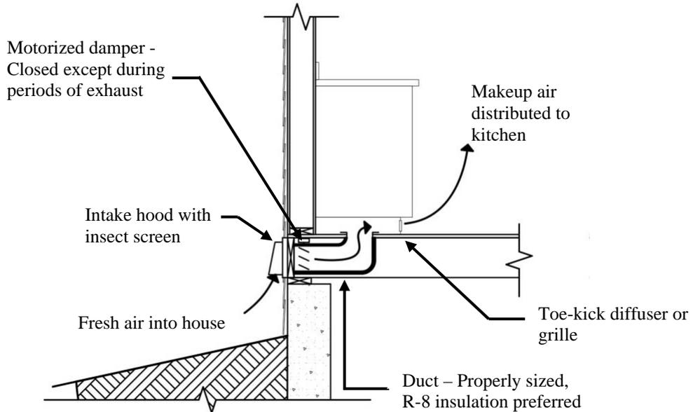
**Figure 2.** Typical engineered opening. The engineered opening in this diagram allows makeup air for a range hood to enter the house into the same room that the exhaust air leaves. This will help to alleviate negative pressure that may result from range hood operation.
