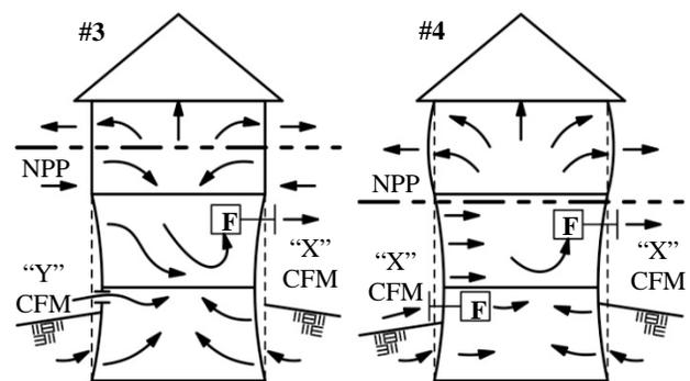
**Figure 1.** Comparison of air movement in a house with an engineered opening (Scenario #3) versus a house with fan-assisted a makeup air system (Scenario #4). In Scenario #3, the neutral pressure plane rises, and the level of house depressurization is less predictable. In Scenario #4, pressures in the house mirror those when no exhaust or makeup air systems are installed (natural conditions).
