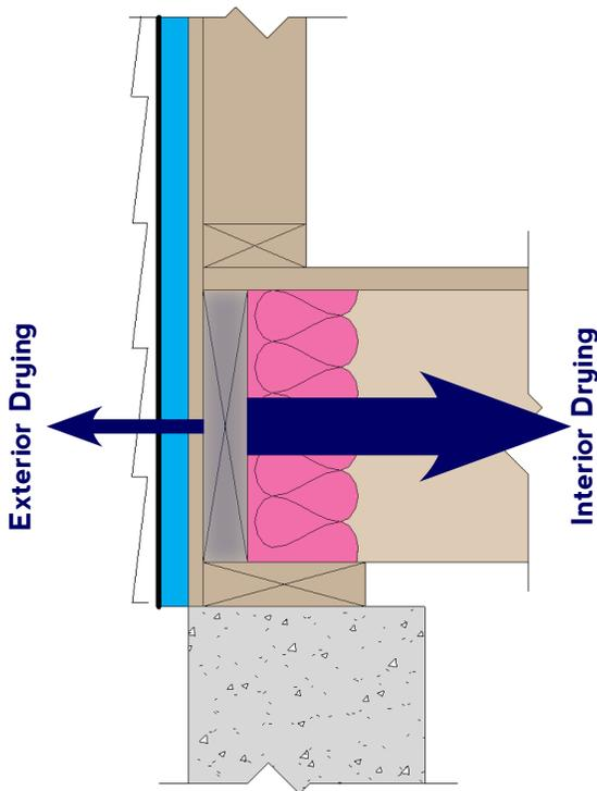
**Figure 4: Rim joist w/exterior foam insulation**
