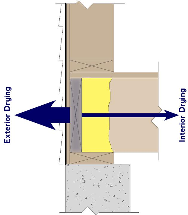
**Figure 3: Rim joist w/interior foam insulation**
