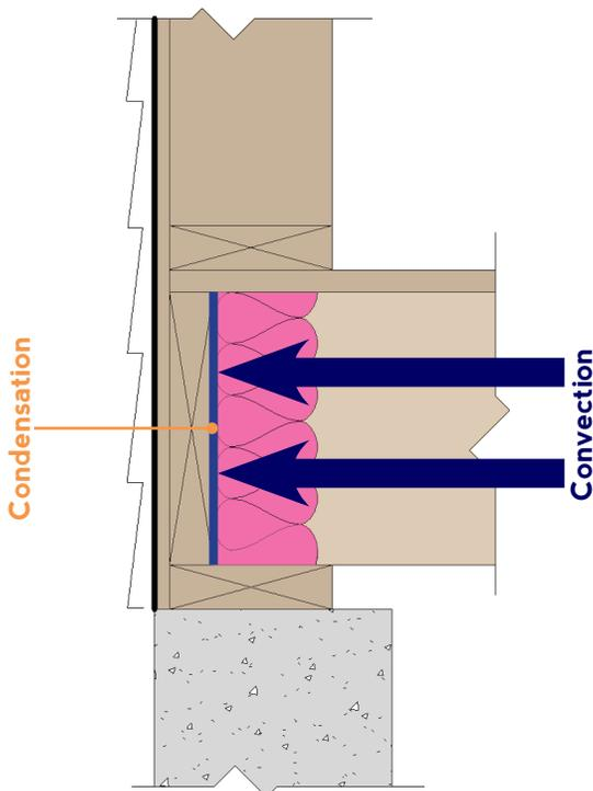
**Figure 2: Rim joist assembly w/fiberglass insulation**
