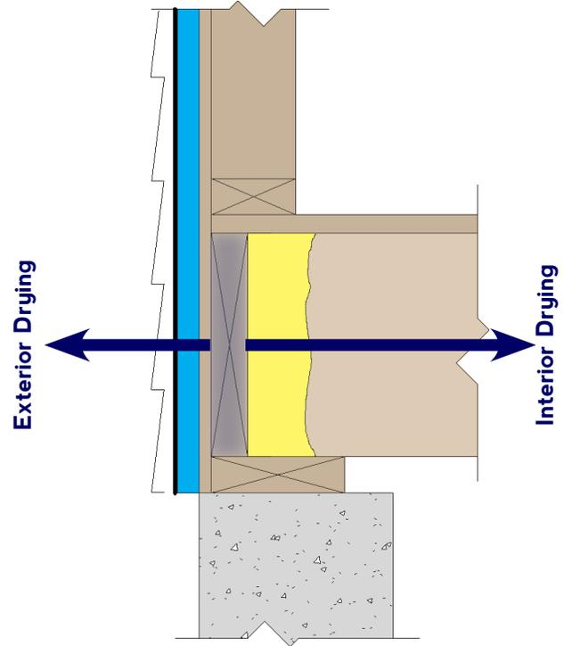
**Figure 5: Rim joist w/interior and exterior foam**
