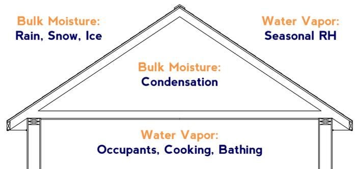
Figure 1: Moisture sources at roof/attic assembly
