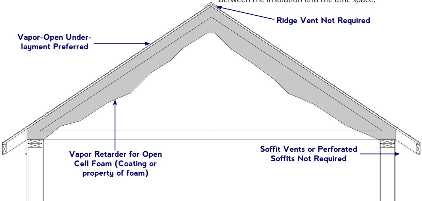
**Figure 4: Critical moisture considerations in unvented insulated roof/attic assemblies using spray foam**
