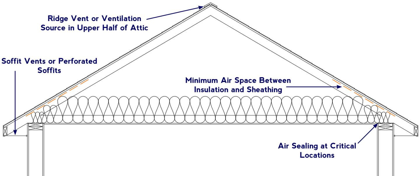
Figure 2: Critical moisture considerations in vented roof/attic assemblies
