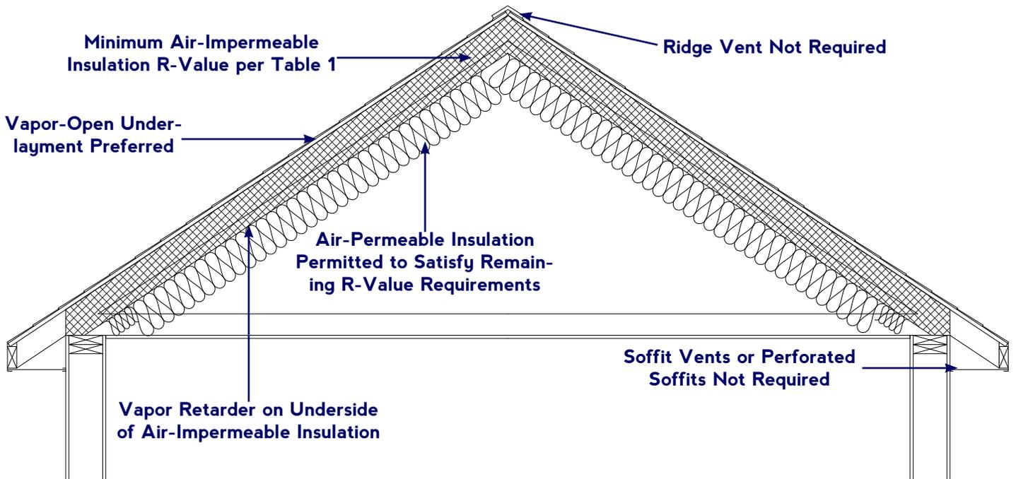
**Figure 3: Critical moisture considerations in unvented insulated roof/attic assemblies using rigid foam**
